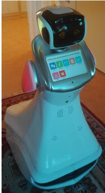
Figure 1. The socially assistive robot (SAR) prototype "Sanbot Elf".
