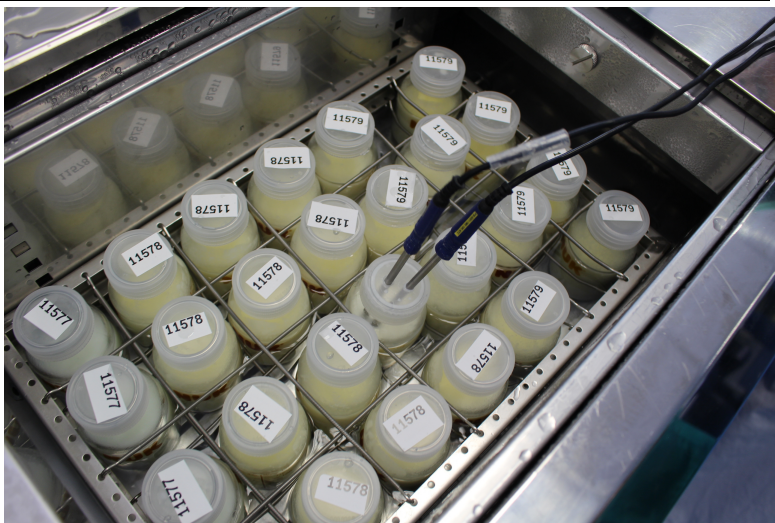
Fig. 3 – Donated human milk bottles at the pasteurizer following the Holder pasteurization protocol at 12 de Octubre HMB (photographed by the authors).
